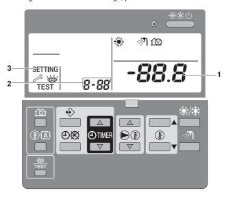
Press the ## button for a minimum of 5 seconds to enter FIELD SET MODE.
